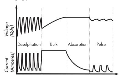
**Desulphation** - Desulphation with pulsing for sulphated batteries.
