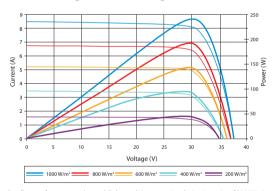
Excellent performance under weak light conditions: at an irradiation intensity of 200 W/m (AM 1.5, 25  $^{\circ}$ C), 95.5% or higher of the STC efficiency (1000 W/m<sup>2</sup>) is achieved
