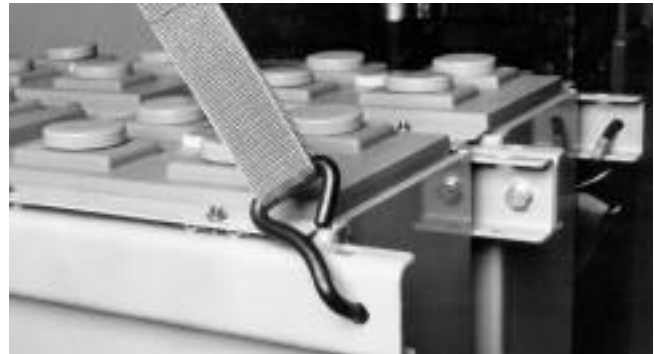
Figure 3: Lifting strap/hook attached to a module
