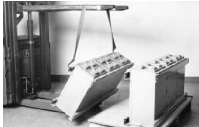
Figure 4: Lifting the module clear of the pallet
